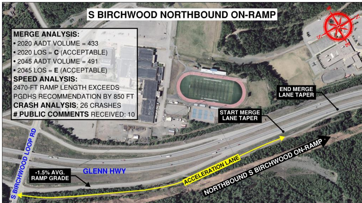
Figure 17. S Birchwood Northbound On-Ramp Location, Characteristics, and Data
