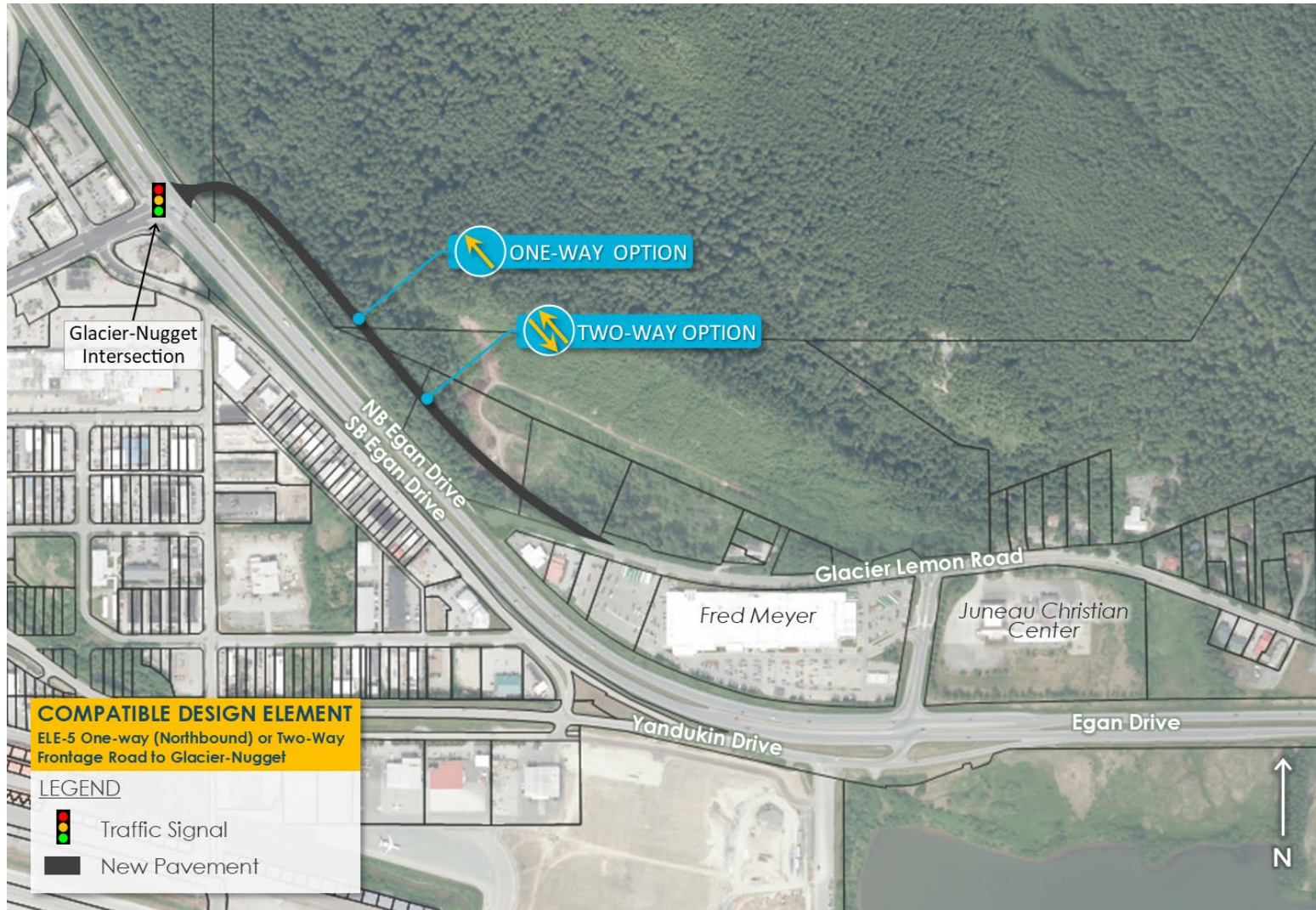
ELE-5. Compatible Design Element: One-way (Northbound) or Two-way Frontage Road to Glacier-Nugget
